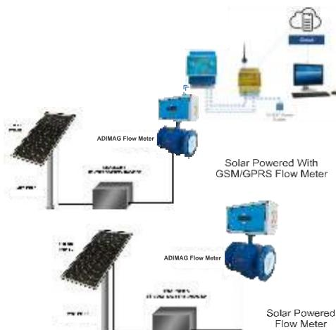
ATN solar powered and GSM/GPRS electromagnetic type flow meter is called TEJMAG300S is battery powered electromagnetic flow meter. It is ideal when power supply on field not present, the battery powered TEJMAG300S gives the flexibility to install a reliable flow meter, virtually anywhere, without distorting accuracy & performance. TEJMAG300S. The flow meter is extremely easy to use, simple to install & requires no regular maintenance.
